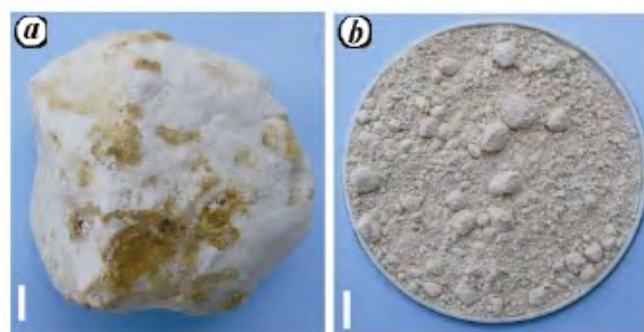
Figure 5. Specimen (a) and powder (b) of hydrous sulphate consisting of minamiite and natroalunite assemblages from Matanumadh, DVP. Scale bar equals 1 cm.
